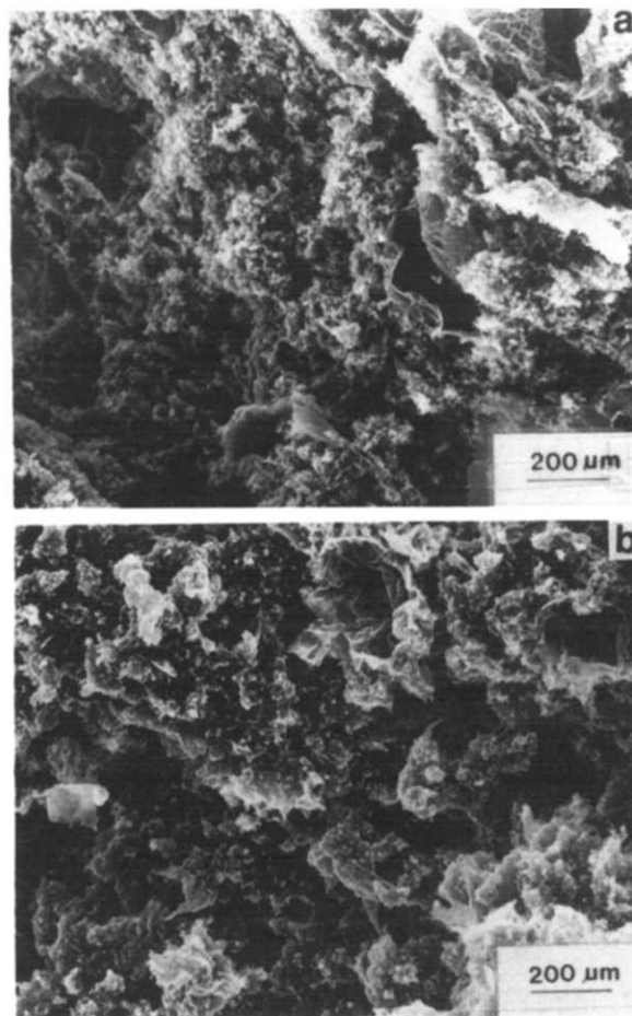
Figure 4 Scanning electron micrographs of (a) polypyrrole/polyurethane/polyacrylamide composite prepared by the concentrated emulsion pathway, and (b) polypyrrole/polyurethane/polyacrylamide composite prepared by the polyurethane solution pathway
